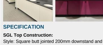
Style: Square butt jointed 200mm downstand and 100mm upstand with thumbnail radius exposed edges. Depth: 300/350mm for semi-recessed basins 600mm for inset basins Material: 13mm solid grade laminate Colours; ref to the Cube colour selector Cut-Outs: Bowl cut-outs are not included unless mentioned separately
